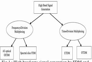
Fig.1 : High baud rate signal generation by FDM and TDM methods reported in previous work
