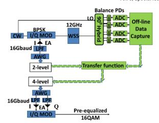
Fig6: The principle of pre- equalization.
