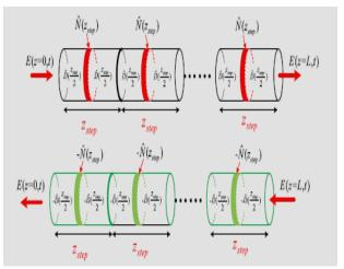
Fig5: The principle of the fiber nonlinear compensation based on digital backward propagation (DBP) method.
