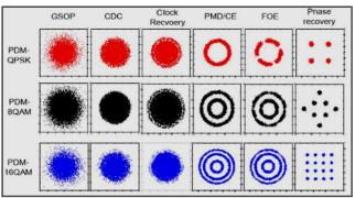
Fig4: The constellation of different signals after 1000-km transmission with DSP
