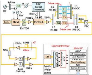
Fig 2: 110 GBaud QPSK signal generation, transmisson and coherent detection system.
