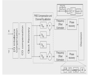
Fig.3: Typical digital signal processing at-the receiver side for coherent optical communication.
